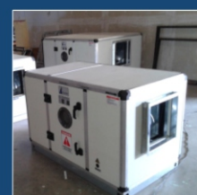
AIR HANDLING UNIT
