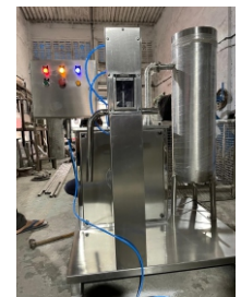
SS Canister Destruction Machine
