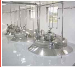
All wetted Parts of SS 316 (cGMP Model) & Pipelines EP Polish
