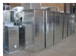
Factory prefabricated ducting
